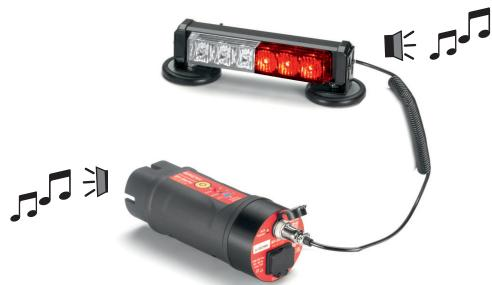
To use the magnetic lashing light, it must be plugged into the rear socket, the beacon can be placed on the vehicle at fault. The LED and buzzer functions described below are **simultaneously** reproduced by the beacon.
